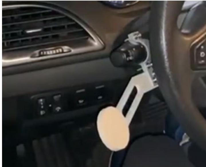
**Fig. 4.** Final product mounted on the blinker. Source: Self-made (Alonso, C. & Santamaría, P., 2022).
