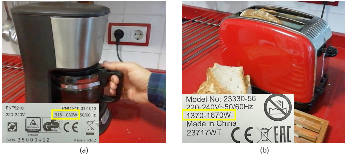
Figure 2.1. (a) coffee maker and (b) toaster, with their technical labels.
